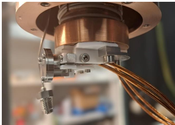
Figure 1: A combined field emission and gas field ion emission source.
